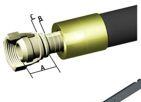
**3.** Push the ferrule onto the hose until it stops. Lubricate the insert and push it into the hose until the stop "B" meets the hose end. Thereafter, pull out the ferrule towards "C".
