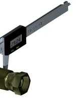
**4.** Swage the ferrule and the fitting according to the required swage diameter (see the Swaging Manual). Use a caliper to check the swage diameter.
