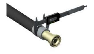
5. Make sure that the correct internal collapse (see the Swaging Manual) has been achieved by using the Hydroscand control pin (9013-xx-xx). The GO side should pass into the fitting to make sure the swaging is not overdone. The STOP side, on the other hand, should not be able to pass to make sure the swaging is not underdone. Please note that on these fittings the STOP side should stop at the interlock!
