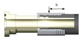
Swage the ferrule's full length with the given swage diameter +2 mm.
