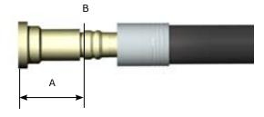
Skive the hose down to the steel wire. The skiving length "L" and "I" is noted in the Swaging Manual. Be careful not to damage the steel wire when skiving. Clean the hose bore from dirt and particles.
