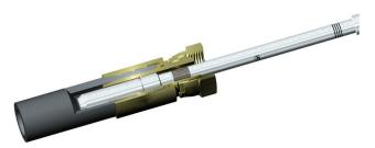
5. Make sure that the correct internal collapse (see the Swaging Manual) has been achieved by using the Hydroscand control pin, 9016-xx-xx.
