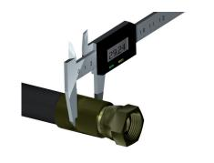
4. Swage the ferrule and the fitting according to the required swage diameter (see the Swaging Manual).
