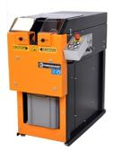
**Product info** TwinSkive is a semi-automatic PLC-controlled skiving machine for external and internal skiving at the same time. The machine can easily reduce your skiving time by 50% and is very reliable and easy to
