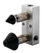
A quick and simple system using compressed air to clean your hose/tube. The tool is delivered with two plastic nozzles, one for hoses and tubes from 3/16" **Product info** to 1" and the other for 1" to 2". Connection: R 1/2" F Product info2 The hose/tube is pressed against the nozzle and thereby opening a valve to allow the compressed air to clean the hose/tube. **Product group** 900 Cleaning Systems Type Length 120 mm Width 50 mm Height 100 mm
